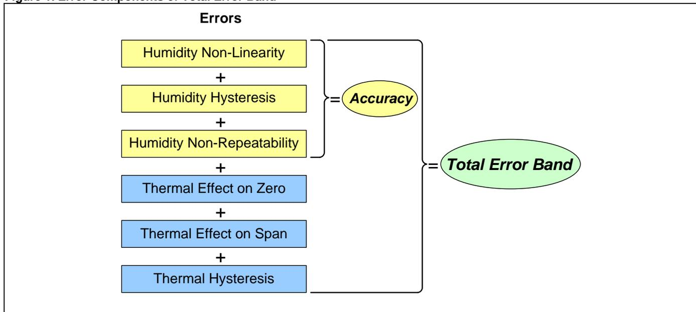
TEB is the maximum deviation from the ideal transfer function of relative humidity over the compensated temperature range and from 10 %RH to 90 %RH (see Figure 2).
