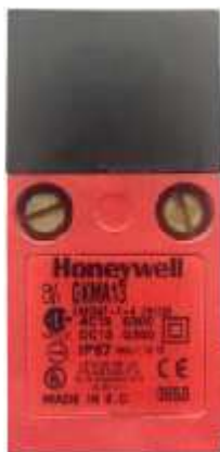
Figure 1: Final Assembly of the GKM-Series Global Miniature Safety Key Operated Switch.
