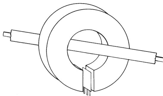
The magnetic field in an electromagnet is not only a function of current, but also of the number of turns on the core. If the current to be measured is greater than 30 amperes, a single turn design can be used, such as shown in **Figure 11**. This type of sensor is particularly useful in high current systems where broad dynamic range, low series resistance, and a linear current measurement are required.
