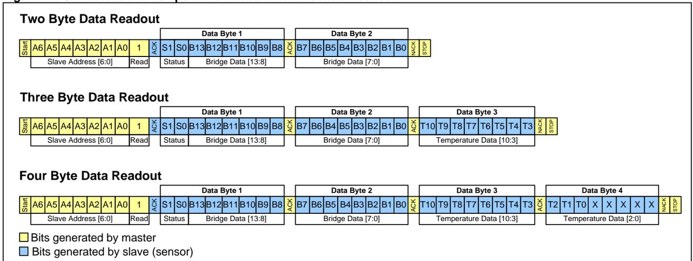
**Note:** For sensors that do not offer the optional compensated temperature output, the sensor will still output the third and fourth bytes of data, but the information contained in these bytes is non-corrected data, and should not be used.
