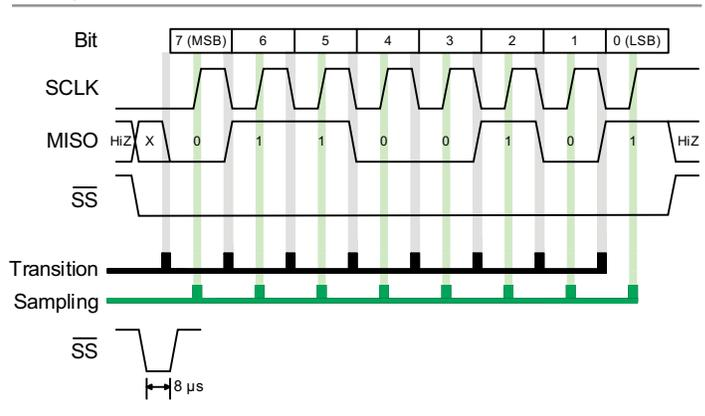
Once the clocking begins, Honeywell digital output force sensors are designed to output up to four bytes of data, depending on the sensor options and application needs. In all cases, the first two data bytes are the compensated force output, along with sensor status bits. The third and fourth bytes are for optional compensated temperature output.
