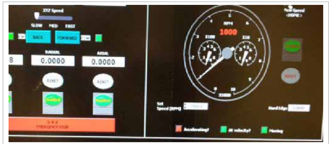
Figure 3. A custom software application was used to precisely control target rotation and sample position.
