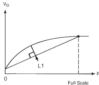
curve. The data point is chosen to achieve the maximum length of the perpendicular line. The length of the perpendicular line represents terminal base linearity error (**Figure 4**).
