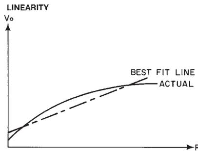
Another method is terminal base linearity (T.B.L.) or end point linearity. T.B.L. is determined by drawing a straight line (L1) between the end data points on the output curve. Next draw a perpendicular line from line L1 to a data point on the output
