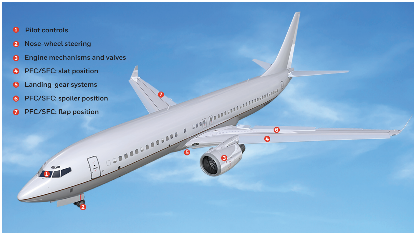
Figure 1. LVDT Position Measurement Applications for Aircraft
