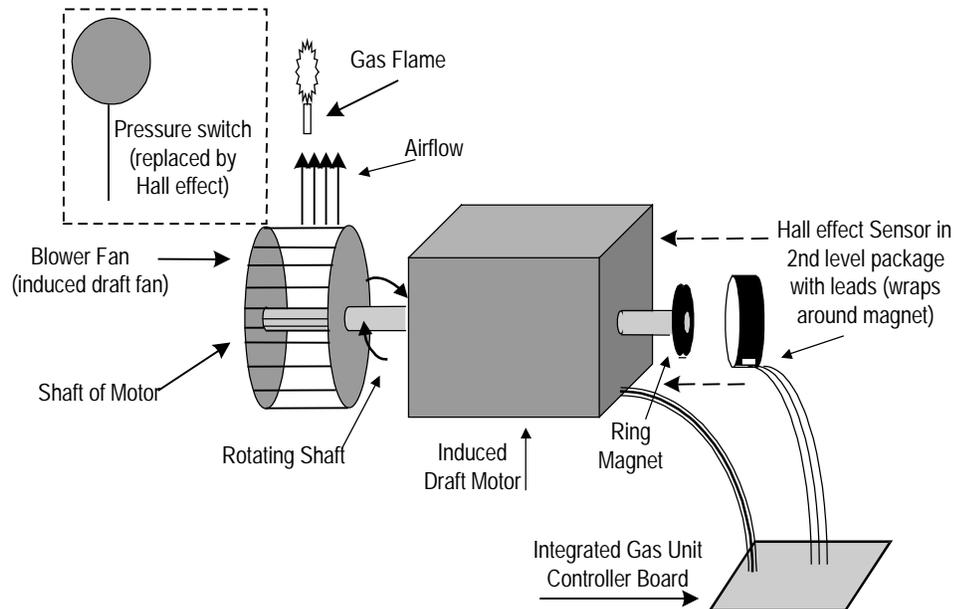
Figure 1. Hall effect sensor in “proof of airflow” application
