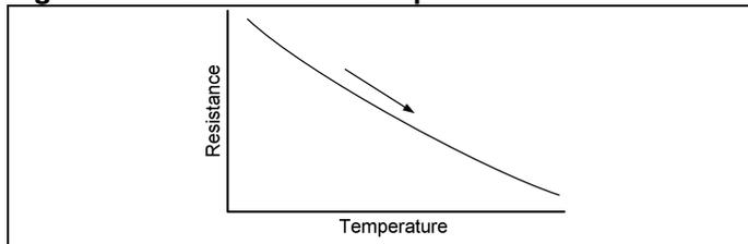
The steepness of the curve is usually referred to as its "slope" which is the relationship of "rise over run" (see Fig. 2).
