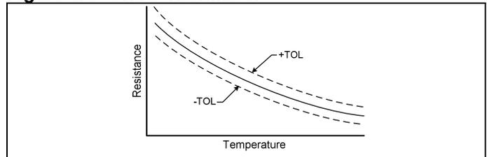
Thermistors that are exactly on nominal (0% at 25 °C [77 °F]) but exhibit slope variations are graphed showing divergent lines, as if the normal curve were rated about the 25 °C [77 °F] point (see Fig. 6).
