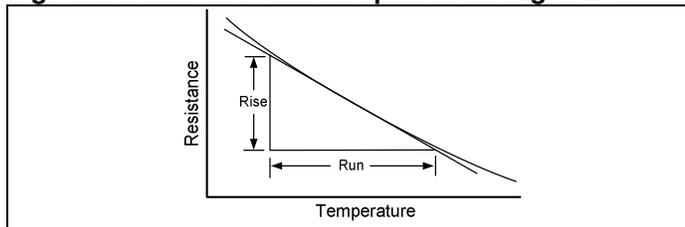
In actual practice, very little data is graphed and analyzed geometrically in this way because it is too time consuming to first obtain sufficient data on a particular thermistor and then to graph the results. It is easier to take resistance data at two widely-separated temperatures and find the ratio of their resistances.
