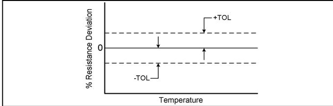
The resistance deviation percentages may also be plotted (see Fig. 8). The result is a horizontal “V” with the point at 25 °C [77 °F]. The V becomes wider with higher temperatures and a mirror image with colder temperatures. A thermistor with a steeper curve and a mirror image with colder temperatures. A thermistor with a steeper curve that is nominal produces the line going down to the right. The upward pointing line results from a thermistor with a less steep curve.
