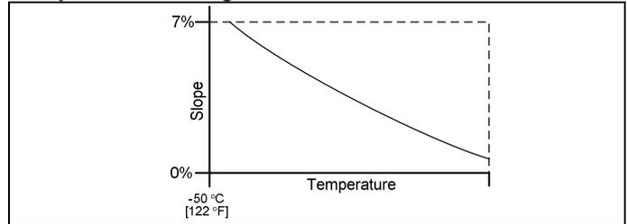
A practical way to find the slope at 75 °C [167 °F] is to use the Steinhart-Hart equation to find the resistance at 74 °C [165.2 °F] and at 76 °C [168.8 °F]. Take the difference in resistance and divided by two. If the slope is required for each degree over a temperature range, then it is most easily done on a computer spreadsheet.
