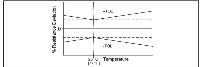
This type of representation resembles a bow tie with the knot at the nominal specification temperature, usually but not necessary, at 25 °C [77 °F]. The tolerance at this point is just the nominal resistance tolerance. To find the tolerance at any other temperature point, the resistance deviation tolerance must be added.
