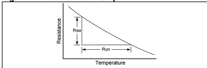
If the graph is quite curved, a straight line is drawn tangent to the curve at the point of interest (see Fig. 3). Also notice that the line slopes "down hill" indicating a negative slope.
