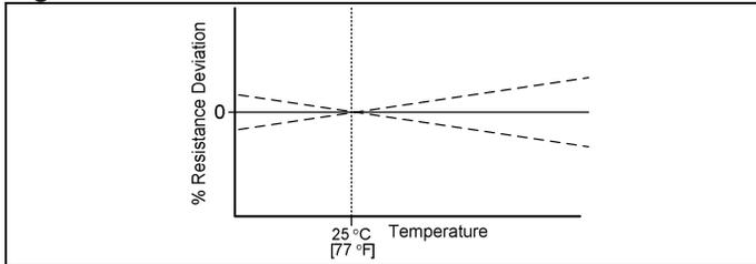
Superimposing the resistance deviation on the plus resistance tolerance and again on the minus resistance tolerance result in the graph shown in Fig. 9:
