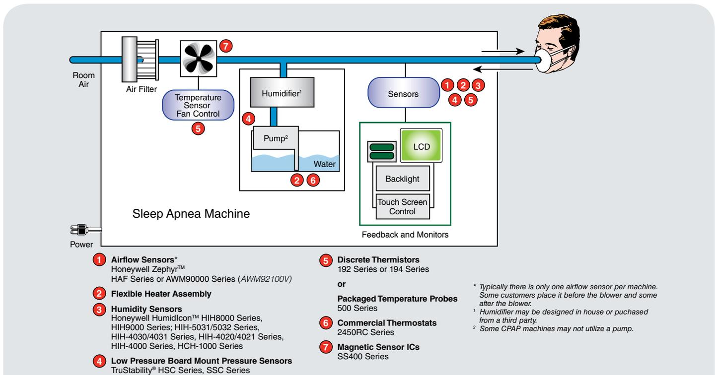
Figure 1. Potential Honeywell products used in sleep apnea machines
